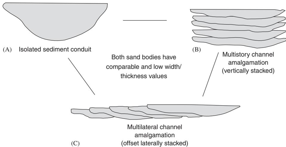
Fig. 6. Generalized variations in channel forms. (A) An erosional channel which may be deep and relatively low aspect ratio. (B) In a confined setting, such as a salt minibasin, channels may stack vertically (i.e., may be multistory). (C) In a less confined setting channels tend to migrate laterally, giving rise to multilateral amalgamation and a higher aspect ratio for entire deposit. Modified from Clark and Pickering (1996).
