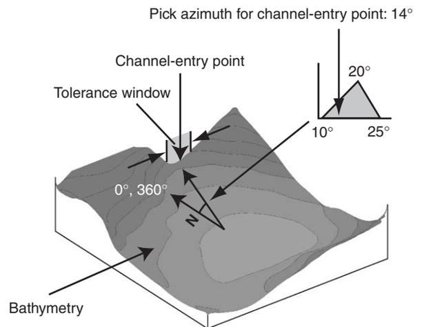
Fig. 3. Schematic diagram that illustrates selection of channel-entry point. Channel-entry point from which a channel reservoir element originates is determined by, first, randomly selecting azimuth for proposed location from an input histogram. Final channel-entry-point location is selected from within a tolerance window surrounding proposed location for channel-entry point.
