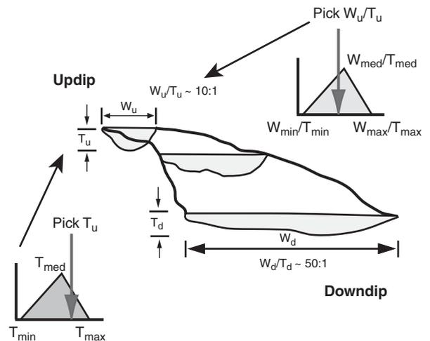
Fig. 4. Schematic diagram that illustrates selection of starting channel thickness and aspect ratio. These initial values are randomly selected from corresponding input triangular histograms. Updip-to-downdip aspect ratios (width-to-thickness ratios) of channel fill a range from as low as 10:1 to approximately 50:1. Channel width increases downdip for all channels. Channel-fill thickness decreases across channel width.
